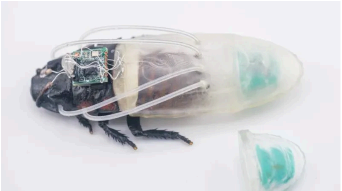
Close-up of the cyborg insect and the new diving suit, which has tubes that connect to the breathing holes of the insect and an oxygen generator mounted at the rear of the suit - NTU Singapore
